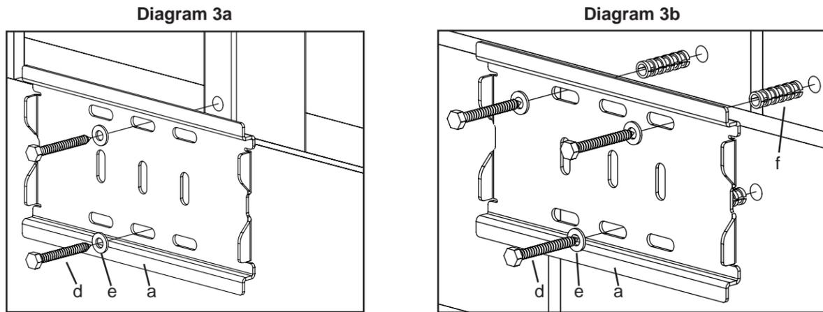
**Step 4: Attach Monitor to Wall Plate**
