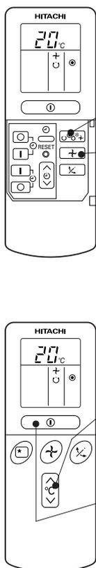
**1** Press the FUNCTION selector so that the display indicates ● (HEAT).
