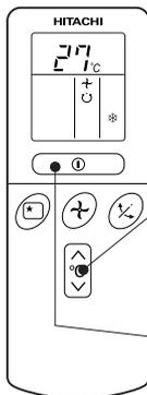
**2** Set the desired room temperature with the TEMPERATURE button (the display indicates the setting).
