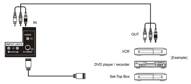
P If your external device has a S-Video terminal, S-Video connection is recommended for higher quality picture.
