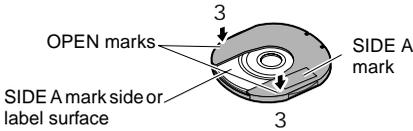
**2** Close SIDE A of the Round DVD Holder, and push it to lock the release levers at positions (3).
