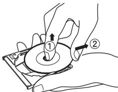
Slide the disc obliquely upward
