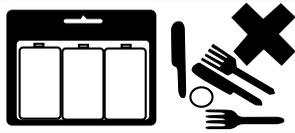
Store unused batteries in their packaging and away from metal objects which may cause a short-circuit resulting in leakage or, in extreme cases, fire or even an explosion.
