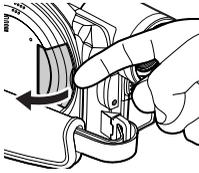
③ Insert the card all the way until it locks, and then close the cover of card insertion block.
