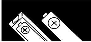
Take care to fit your batteries correctly, observing the *plus* and *minus* marks on the battery and appliance. Incorrect fitting can cause leakage or, in extreme cases, fire or even an explosion.
