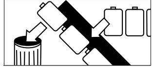
Replace the whole set of batteries at one time, taking care not to mix old and new batteries or batteries of different types, since this can result in leakage or, in extreme cases, fire or even an explosion.
