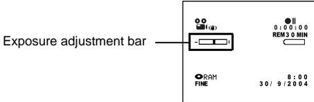
**2** Use the  $\ominus$   $\oplus$  buttons to adjust the exposure, while viewing the image in the viewfinder or on the LCD screen.
