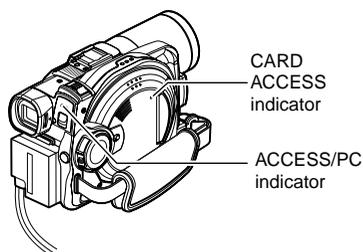
If you turn the DVD video camera/recorder off while the ACCESS/PC or CARD ACCESS indicator is lit or blinking, turn it on again with the disc or card loaded in it: Repair of the disc or card will be executed automatically (see page 168).
