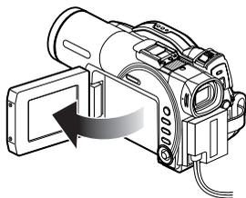
② While holding the grey switch at the centre of power switch, set the switch to "CARD PHOTO".
