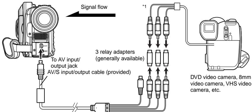
\*1: The AV/S input/output cable provided with this DVD video camera/recorder can be directly connected to some video cameras.
