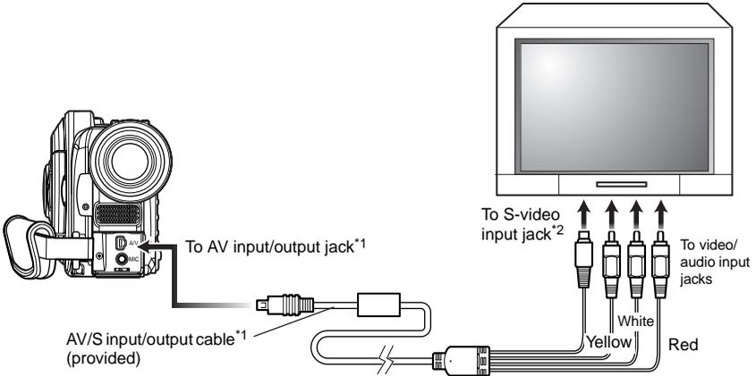
\*1 AV/S output cable and AV output jack for DZ-MV550E (UK) and DZ-MV580E (UK): External input is not available on these models.
