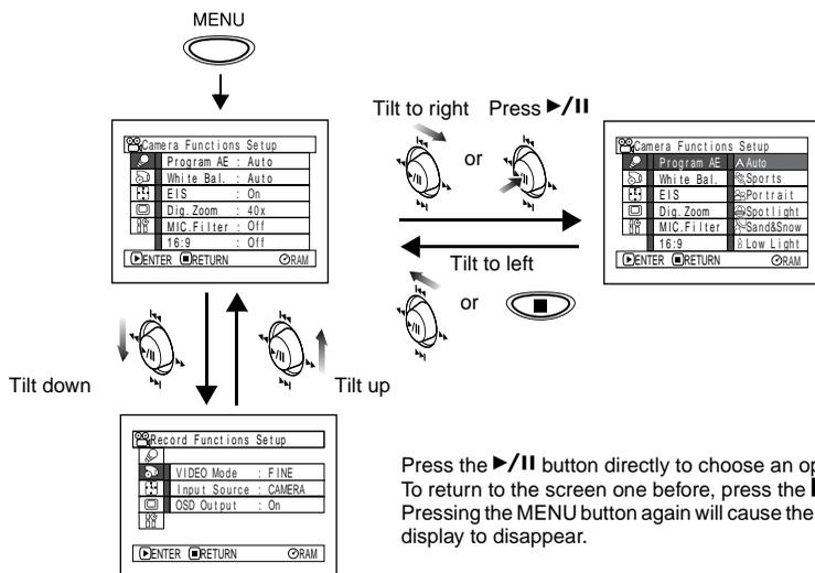
Press the >/|| button directly to choose an option from menu. To return to the screen one before, press the ■ button. Pressing the MENU button again will cause the Normal mode display to disappear.
