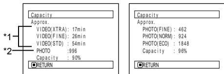
\*1 With DVD-R disc: The quality mode first used for recording with disc will appear.
