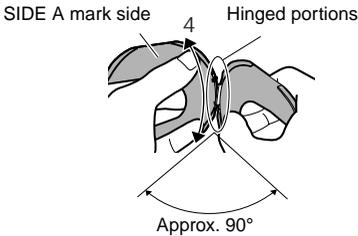
**2** Fit the hinged portion of the other holder piece into the warped hinge portion.
