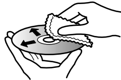
Use the disc cleaning cloth to clean from inner to outer edges in axial direction.
