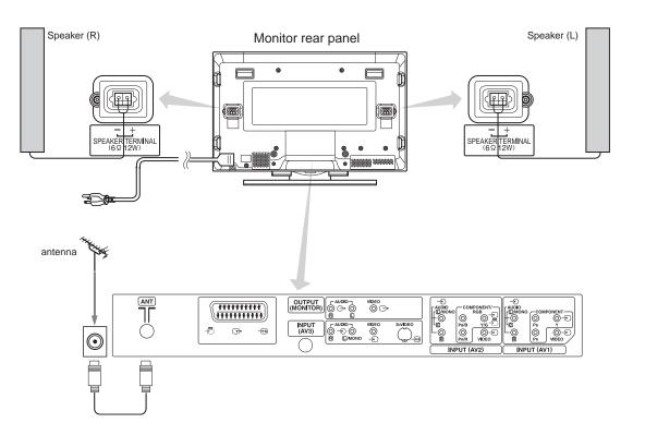
When the "ANT" terminal is connected to outdoor antenna instead of CATV system, please note that a good antenna adaptor is necessary. See the diagram on the right.
