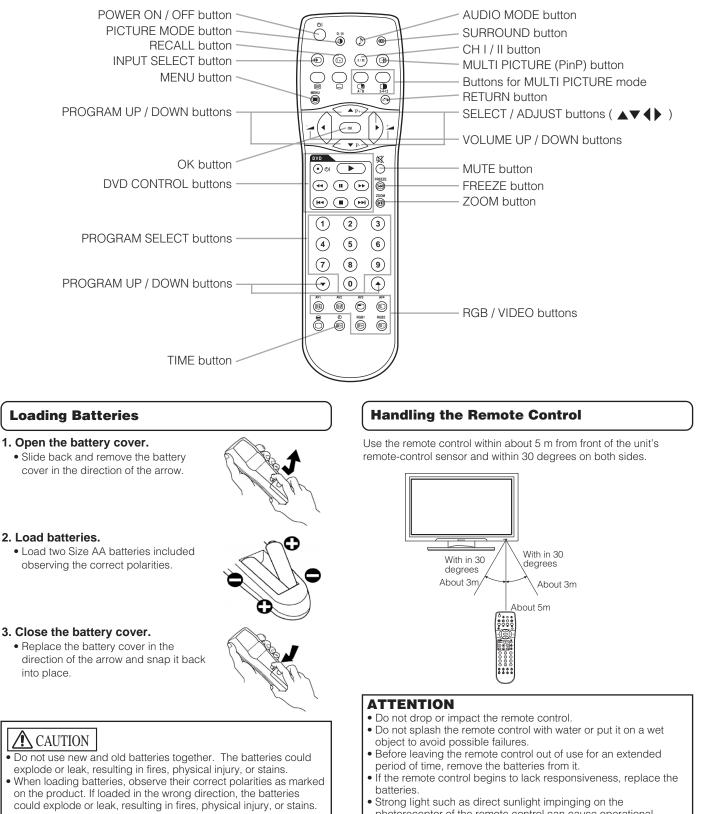
Strong light such as direct sunlight impinging on the photoreceptor of the remote control can cause operational failure. Position this unit to avoid direct contact with such light
