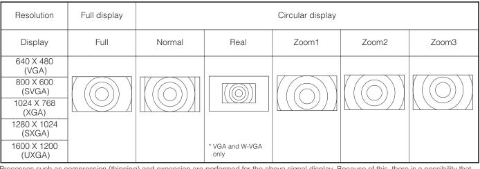
Processes such as compression (thinning) and expansion are performed for the above signal display. Because of this, there is a possibility that flicker may become noticeable on Zoom  $(1 \sim 3)$  depending on the display contents. If this occurs, turning the Vertical Filter On 20 can reduce the flicker.
