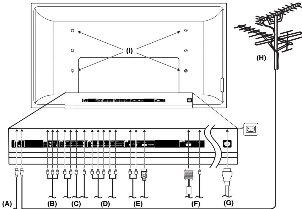
**(A) Antenna connection:** The built-in Hyperband CATV tuner can receive all analog cable television programs.
