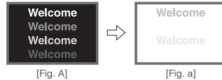
■ The degree of image retention is proportional to the brightness of the characters and figures displayed as well as the display time.
