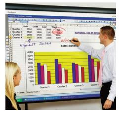
The new wireless connection option from Hitachi overcomes the 5 metre length restriction for USB connections as the wireless USB server connects directly to the FX-Duo Board using the whiteboard's existing USB lead. A separate wireless adaptor connects to the controlling computer's USB port which will then establish two-way communication to the board via the wireless server providing an instant wireless connection between the computer and the whiteboard.
