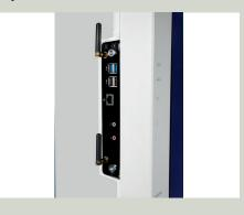
The option of an integrated PC means your Hitachi IFPD is ready to use the moment it is switched on; no waiting for the panel to turn on, no complicated technical set up or fiddling with cables, it is always available to use, just when you need it. Furthermore, the integrated PC is Bluetooth enabled for use with headsets, mouse or keyboard.
