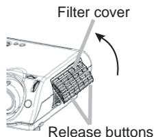
**4 Hold the release buttons of the air filter, while pulling down it.**
