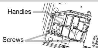
**6 Insert the new lamp, and tighten the 2 screws firmly to lock it in place.**
