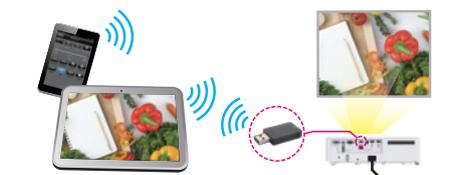
\*This picture shows an example of network connection using optional wireless adapter.
