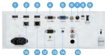
1.HDMI 1 2.HDMI 2 3.HDMI 3 / MHL 4.MONITOR OUT 5.COMPUTER IN 6.VIDEO 7.3D SYNC 8.SERVICE 9.USB POWER 10.RJ45 11.HDBaseT 12.RS-232C 13.AUDIO OUT 14.AUDIO IN 15.AUDIO IN (L/R)
