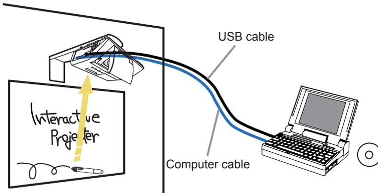
Interactive Function enables interactive operations, such as operation of the connected computer and writing on the screen using the “StarBoard Software”, by making use of the built-in sensor of the projector and the supplied pen without the need of a special board.
