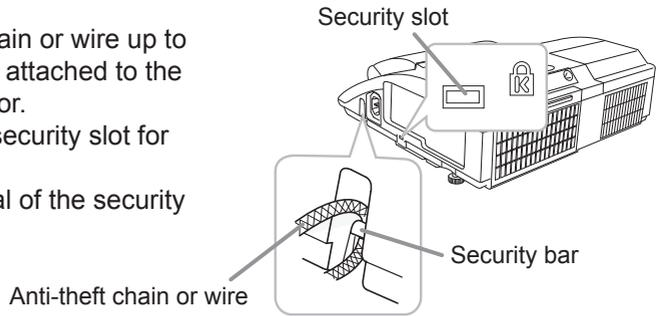
**⚠ WARNING** ► Do not use the security bar and slot to prevent the projector from falling down, since it is not designed for it.
