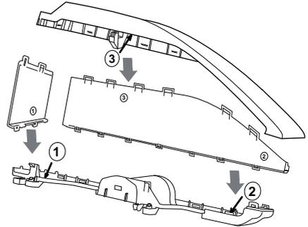
3. Insert the three knobs on the cable cover into the three holes on the projector as shown in the figure. Pass the cables through the holes on the bottom of the cable cover.
