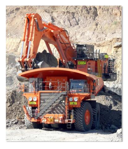
Putting production figures of the two 550-tonne excavators on site against each other provides for an interesting comparison. The EX5500 performed to NRW's planned dig rates. However, according to Shaun Lucas, the EX5600 excavator, matched with the EH4000 trucks, provided "about 30% in end-yield on top of what the 5500 does".
