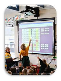
The Hitachi CP-A100 Ultra Short Throw Projectors are appealing to Margate staff as the shadow effect is severely reduced, allowing the Starboards to be used at close range. The projectors are able to produce a 60 inch image when installed only 9.6cm away from the projection surface and as such, teaching staff have identified the increased engagement of students within the learning environment as a highlight.
