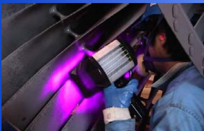
LP Turbine Rotor Non-Destructive Testing
