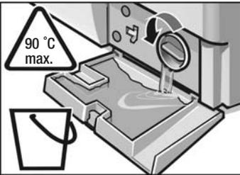
3. Unscrew the pump cap **slightly** until the washing solution slowly begins to run into the cover plate cavity.
