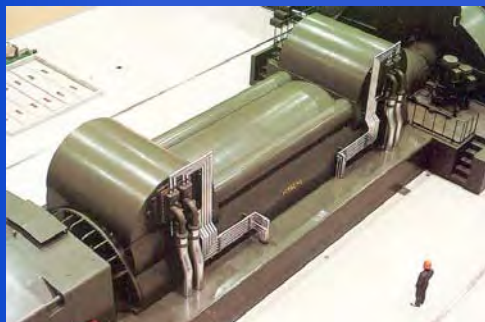
1,300 MVA Nuclear Turbine Generator, Japan
