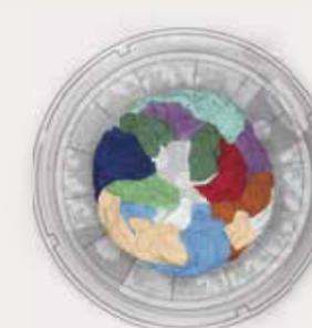
The pulsator repeatedly moves clockwise and counterclockwise to make items fall off the tub wall.
